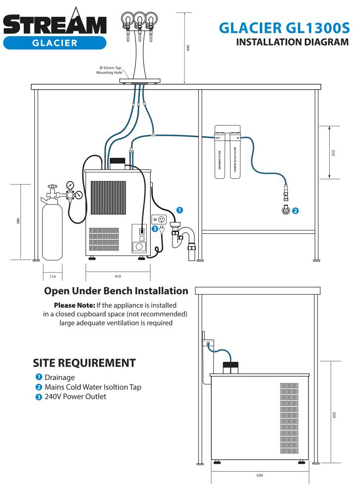
**N.B.** When trimming tubes to length - to ensure NO LEAKS use a sharp tube cutter for a clean cut
