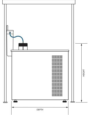
**N.B.** When trimming tubes to length - to ensure NO LEAKS use a sharp tube cutter for a clean cut ALL DIMENSIONS GIVEN ARE IN MM.
